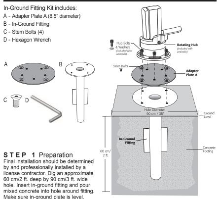
**Note:** Do not get slurry in the screw threads. Either apply tape over the holes on both sides of the fitting or place the stem bolts in the threads and remove them when the concrete is almost set. To make the adapter plate flush with the concrete, recess the inground fitting 3/8" below the finished surface.
